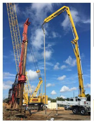
Replace last boom section with Tremie Boom section to increase boom tip load for piling application
