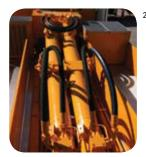
A convenient switch of hoses using the optional SBU rod/piston conversion system allows the user to go from the rod side to the piston side quickly and easily. Capable of pumping pressures up to 3,200 psi (220 bar) on the piston side, the CP 2110 HP can handle a range of applications including high-rise jobs.
